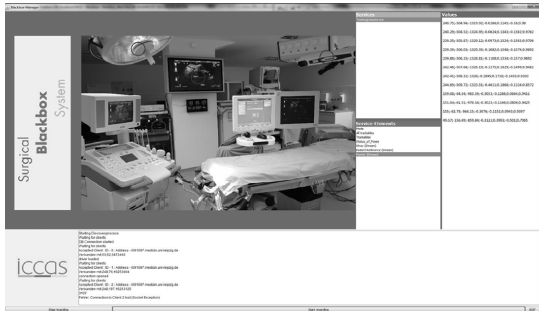
Figure 6.2.2: Prototype of the surgical black box system that might be used e.g. for automatic documentation of the intervention for quality management purposes.
