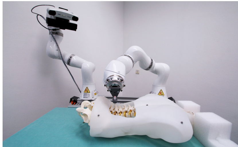
Fig. 1- Scorpio demo setup. Combined tracking system on the left, needle placement system on the right.
