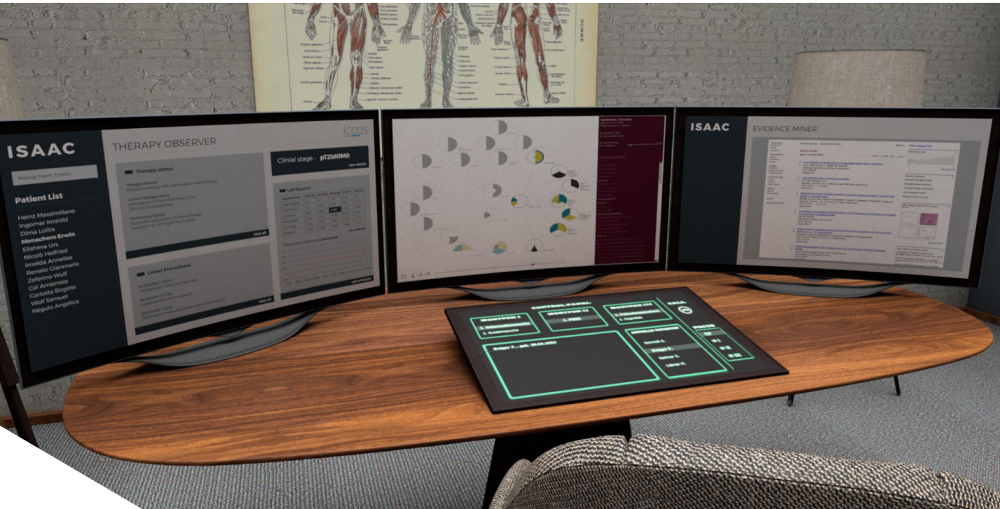
Fig. 1- ISAAC hardware arrangement with curved displays for a broader viewing angle and touchscreen input.
