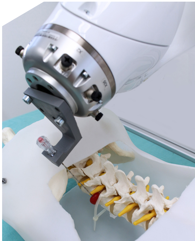
Fig. 2- Needle placement robot holding needle in position at target structure.
