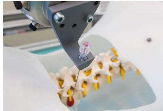
Fig. 2- Robot arm with 3D-printed needle placement end effector.
