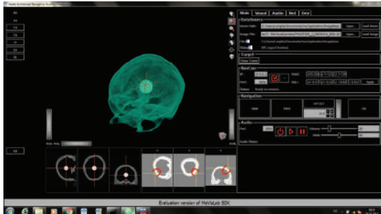
Fig. 2 - Screenshot of the planning step performed by the developed software tool. A model of skull and brain tumor is depicted in green. The surgeon indicates with the pointer (yellow cross) the optimal angle to reach the tumor. Then, the tumor is projected on the skull (small images on the lowest part of the screen). The projection is used to suggest a position for the craniotomy section line.
