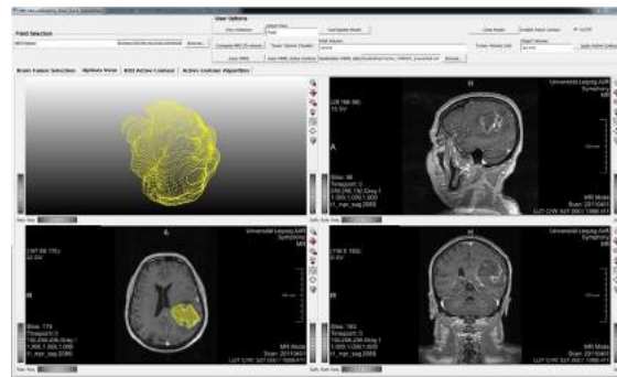
Fig. 1 - Interface of the segmentation tool implemented with MeVisLab. The brain tumor boundary was manually delineated in a couple of slices in the axial view of the preoperative MR data (lower left panel). A 3D tumor model was generated by interpolating the contours between the slices (yellow contours in the upper left panel).
