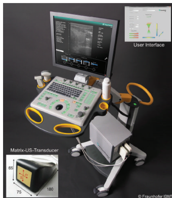
Fig. 2- LIFUP-System with Matrix-Transducer and UI (Fraunhofer IBMT, St. Ingbert).
