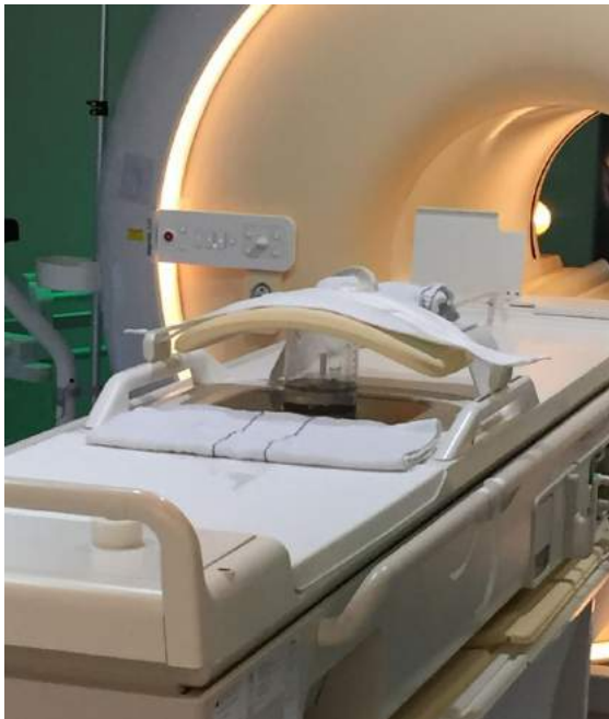
Fig. 3 - Clinical HIFU system (Profound medical) with transducer installed in the tabletop integrated into 3T achieve MR scanner (PHILIPS) at University Hospital Leipzig. Beaker with tubes for hyperthermia treatment stands on the transducer window.
