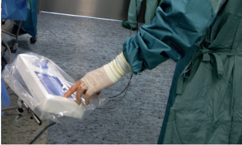
Left: The sterile surgical control console with touchscreen provides access to primary device functions of the integrated OR system. Right: Review and selection of images acquired during intervention for postoperative documentation.
