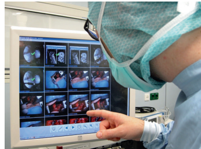
Left: The sterile surgical control console with touchscreen provides access to primary device functions of the integrated OR system. Right: Review and selection of images acquired during intervention for postoperative documentation.
