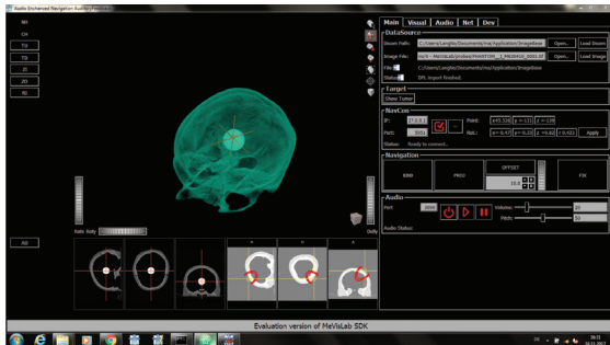
Fig. 2 - Screenshot of the planning step performed by the developed software tool. A model of skull and brain tumor is depicted in green. The surgeon indicates with the pointer (yellow cross) the optimal angle to reach the tumor. Then, the tumor is projected on the skull (small images on the lowest part of the screen). The projection is used to suggest a position for the craniotomy section line.
