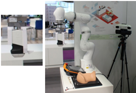
Fig. 1 - The Scorpius robotic system. Shown are the KUKA robot arm, the Clarius L7 wireless ultrasound probe, the tracking camera system and the neck phantom.
