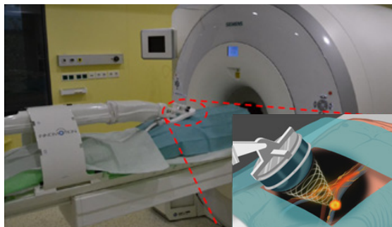
Fig. 2 - Setup of the robotic arm system in the MR-PET system in the Department of Nuclear Medicine of the University Medical Center Leipzig. The robotic arm (left) positions the US transducer according to the planned treatment. The MR-PET system monitors the position of the transducer, the temperature and the efficacy of the treatment.
