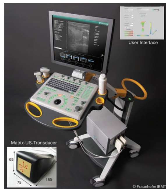
Fig. 1 - LIFUP System with Matrix Transducer and UI (Fraunhofer IBMT, St. Ingbert).
