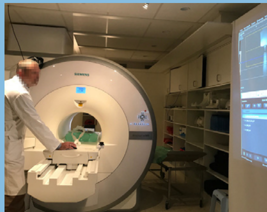
Magnetic resonance (MR) interventional interaction setup at Nuclear Medicine Clinic of Leipzig Medical Center, which allows direct control of the scanner by the physician.
