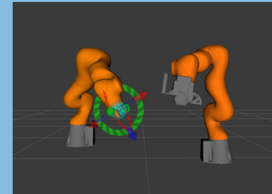
Concept for clinical translation of FUS and RT. Two Kuka robotic arms holding therapeutic transducer and imaging transducer.
