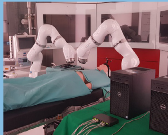
The setup of two KUKA lbr iiwa 7 R800 robot arms (KUKA AG, Augsburg) in the demonstrator OR at ICCAS Leipzig. Robots connected with IEEE 11073 SDC standard.
