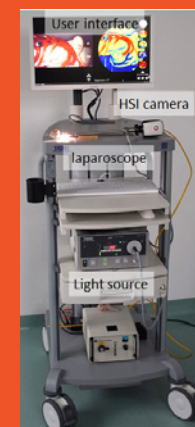
LYSIS laparoscopic HSI system including the miniaturized HSI camera, the laparoscope with light source and the developed user interface.
