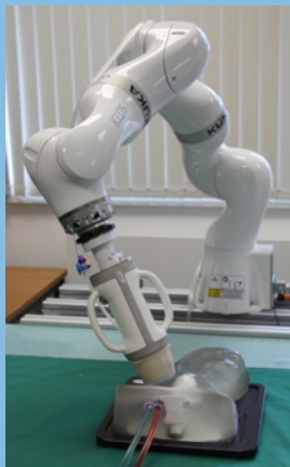
Prototypical system consisting of a Kuka LBR iiwa robotic arm with the treatment head attached.
