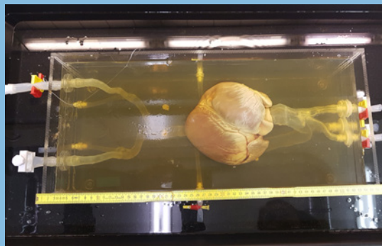
In vitro model for experimental testing of MR guided minimally invasive interventions. Consisting of arterial vessel system (silicone) connected to porcine heart, embedded in gelatin.
