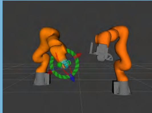
Concept for clinical translation of FUS and RT. Two Kuka robotic arms holding therapeutic transducer and imaging transducer.
