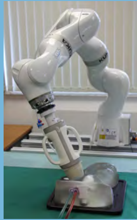
Prototypical system consisting of a Kuka LBR iiwa robotic arm with the treatment head attached.
