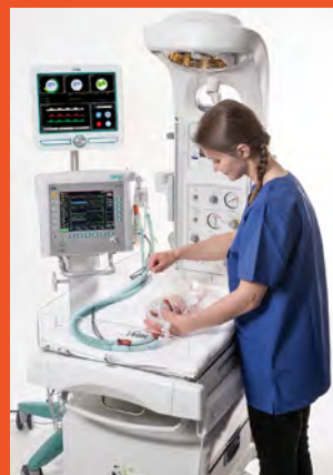
Image of the demonstrator of the future EMU system, on the left the joint system of mechanical ventilator and EIT device is shown connected to an incubator setup.
