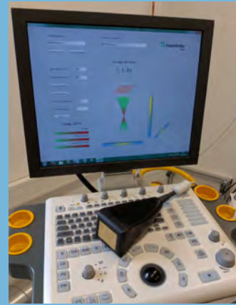
Custom-made ultrasound system (Fraunhofer IBMT) that can be synchronized with EEG recordings
