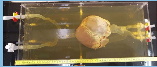
Silicone arterial vessel phantom with a connected porcine heart for ex-vivo studies.
