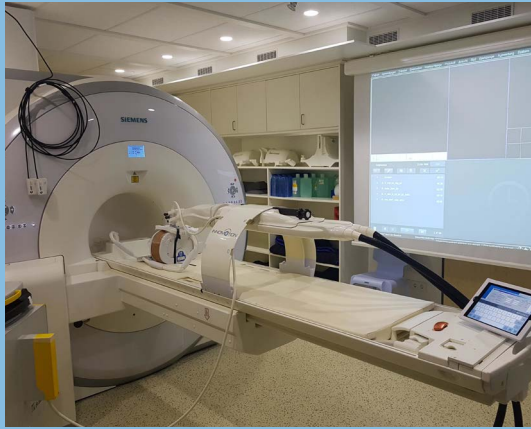
Experimental interventional MRI interaction setup at Nuclear Medicine Clinic of University Hospital Leipzig, which allows direct control of the scanner by the physician.
