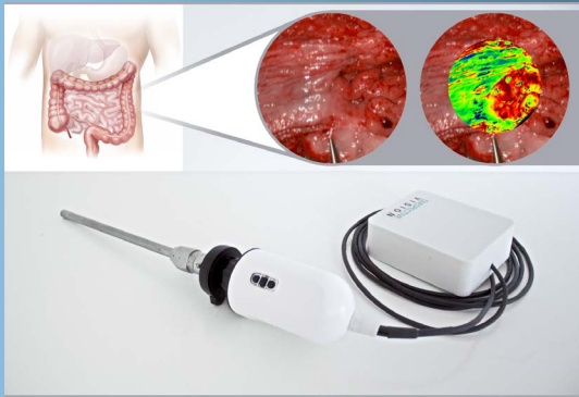
Prototype of the compact laparoscopic HSI system (bellow) and hyperspectral parameter image automatically registered the with the colour video (above right).
