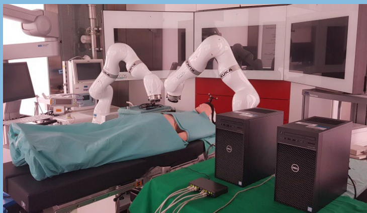
Fig. 2: The setup of two KUKA lbr iiwa 7 R800 robot arms (KUKA AG, Augsburg) in the demonstrator OR at ICCAS Leipzig.
