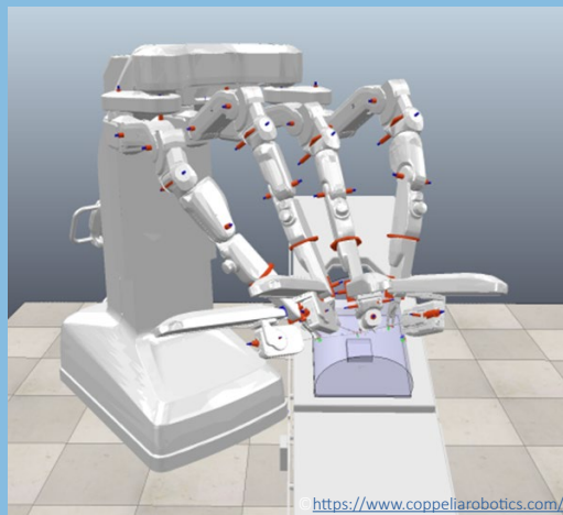
Fig. 3: The avatera robot model in the simulation environment CoppeliaSim.
