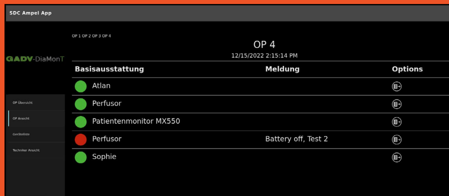
Fig. 13: Visual representation of an OR with attached devices and their technical status. The perfusor is not ready for use (red status and error message).
