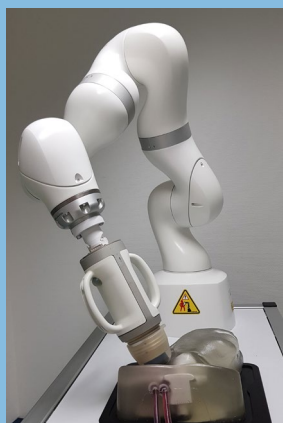
Fig. 1: Prototypical system consisting of a Kuka LBR Med robotic arm with the treatment head attached.
