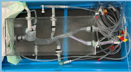
Fig. 6: Silicone-based patient model for simulation of MRI-guided vena cava filter (VCF) delivery with implanted VCF with introduced in-vitro thrombus (white arrows).
